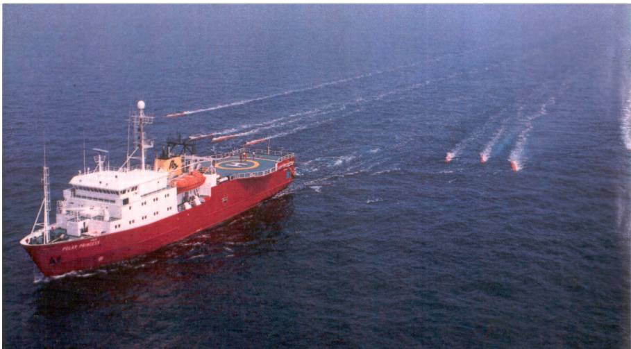
FIGURE 1.5. Seismic survey vessel towing a number of hydrophone arrays
